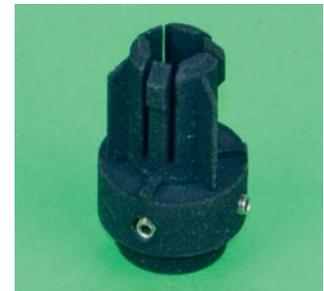
Spare parts, fabricated using 3D-printing
